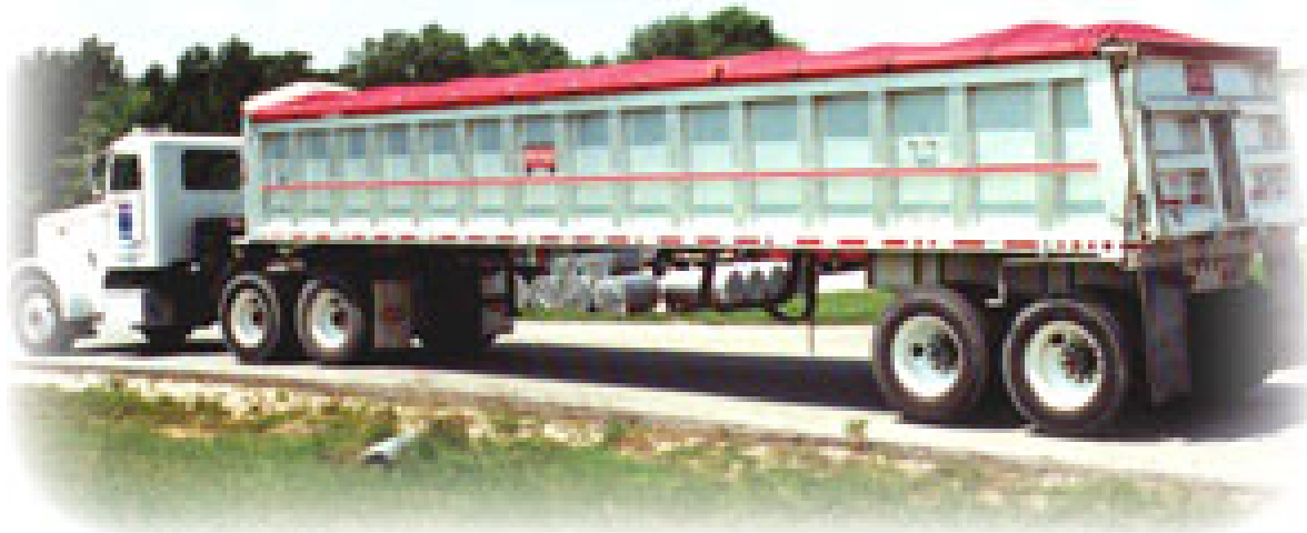
Figure 1 - This is an example of a five axle vehicle with two sets of consecutive tandem axles. The truck tractor has a single axle in front with a set of tandem rear axles. It is pulling a trailer with a set of tandem axles.
