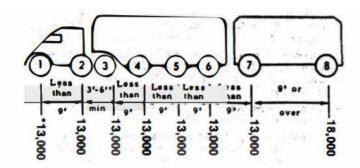
Because axles 1 through 7 are less than nine feet but more than three and a half feet away from each other, their maximum allowable gross axle loadings are 13,000 pounds. Axle 8 is at least nine feet from axle 7. As such, its maximum allowable gross axle loading is 18,000 pounds.
