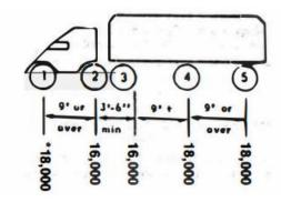
Axles 2 and 3 are part of a tandem axle assembly. As such, their maximum allowable gross axle loadings are 16,000 pounds. Because axles 1, 4, and 5, are at least 9 feet away from another axle, their maximum loadings are 18,000 pounds.
